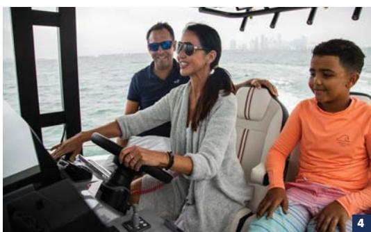
**4. PROTECTED HELM STATION** The extra-wide console is protected on three sides by windshields and has abundant room for twin multifunction displays, with steering and engine controls close at hand. Plus air conditioning really cools down the helmsman and crew. Overhead, a standard hardtop offers sun protection and is equipped with a sliding hatch for additional ventilation. Here, too, five fishing rod holders can be mounted.
