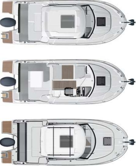
**1. MULTIPURPOSE COCKPIT** The aft cockpit features optional U-shaped bench seating that transforms into a large sundeck. The rear bench slides forward enabling the engine to be fully raised while still being able to enjoy the cockpit seating.
